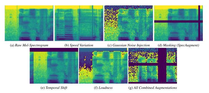
Figure 1: Examples for transformed mel-spectrograms, that are used in model training as given in section 3.
